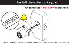
Align the exterior keypad with the bore hole. Feed the power cable through latch The spindle on the exterior keypad should be aligned with the hole in the center of the latch. Insert the spindle through this hole as you press the exterior keypad
